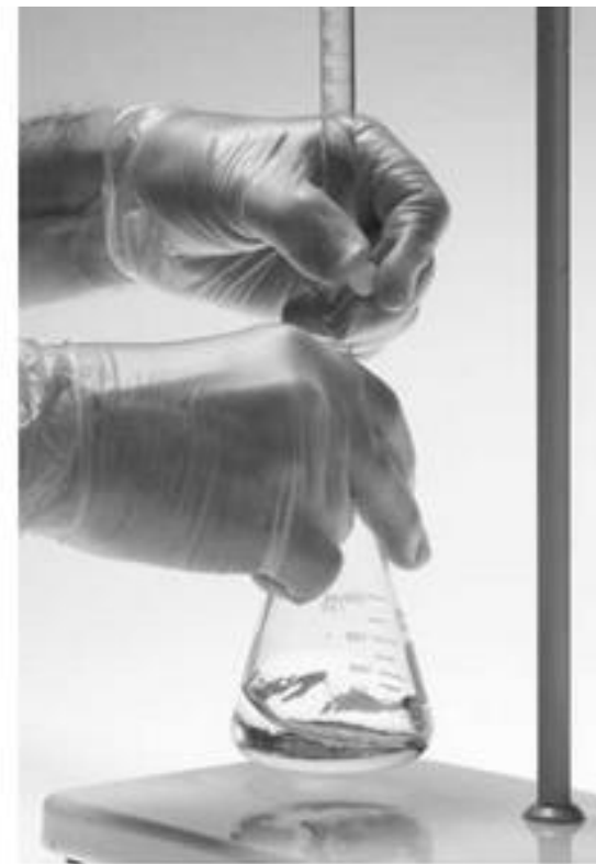
Figure 2-23 Recommended method for manipulating a buret stopcock.
